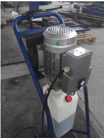
**Step3, Connect fitting and oilhose from engine to piston.**
