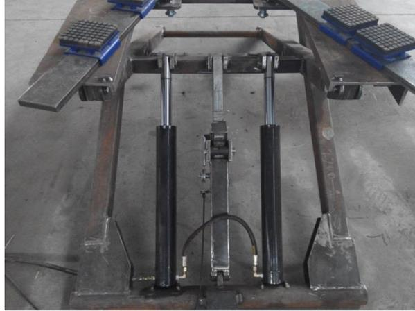
**Step 5, Mount the lock releasing wire**
